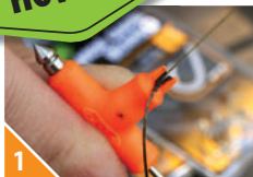
1 Start by cutting 12ins of Camotex Semi-Stiff and strip away 4ins of out coating from one end
